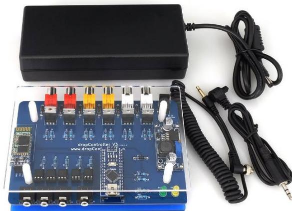
Includes dropController, power supply, shutter release cable, flash trigger lead. The shutter release cable shown has been replaced with a coiled type.
