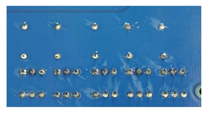
This can be cleaned up using Isopropyl Alcohol, a small brush (old tooth bush is fine), and some elbow grease.
