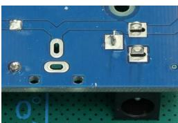
Partially solder one pin and check the socket hasn't moved.
