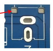
Double check that you have the socket in the correct position and that they are flush with the PCB before soldering. The should have a fairly tight fit so once you have them in the right place they should stay put while you solder them.
