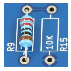
When the pins have rounded corners the resistor sits in the middle where it belongs
