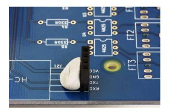
Place the header and fix it in place with the Blutack
