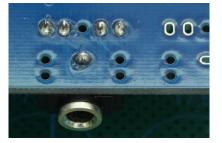
Make sure the socket is flush to the PCB. The pins should be fully through the PCB and the small tabs on the bottom of the sockets should be in the 4 holes.
