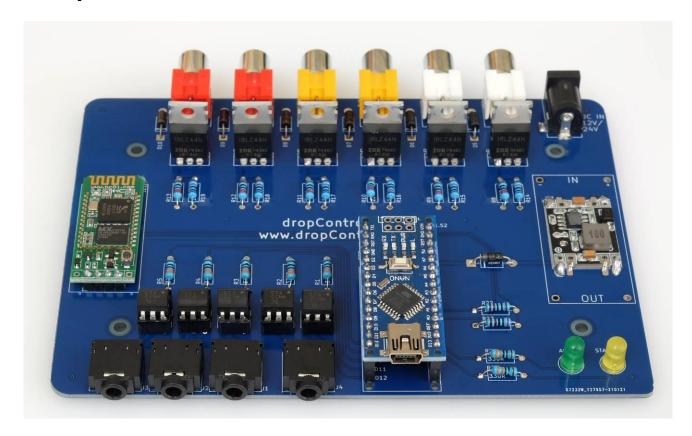
PCB v1.52 with the 9v DC-DC buck converter.
