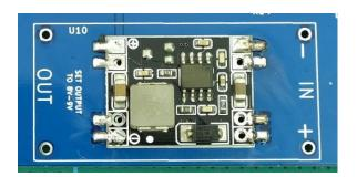
Heat up the pad on the PCB and then solder in place by running solder from the pad on the PCB to the pad on the converter.
