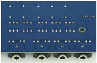
Double check that pins are not joined together.
