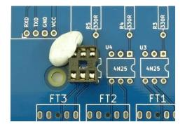
Getting the socket to stay in place when you flip the board over can be finicky. A small blob of Blutak can help. When soldering you want enough solder to hold the pins but not so much that you cause a flood and join all the pins together. Place one socket, flip the board over, solder a corner pin, check the position, and if the socket is still in place, solder the remaining pins.
