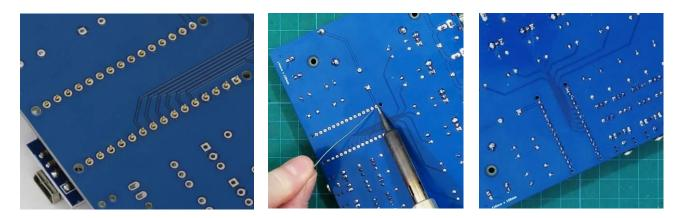
Solder one corner then check that the headers are still in position and are lying flat. Solder the opposite corner and check again.
