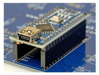
Solder the Arduino pins.
