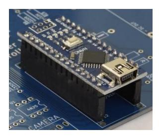
After soldering the Arduino pins, flip the PCB upside down and solder the headers to the PCB
