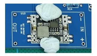
I like to hold the buck converter in place while I attach it.
