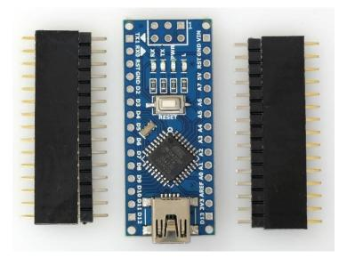
Start by inserting the Arduino pins into the headers
