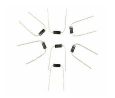
As with the resistors, bend the legs from the end of the leg so you get a nice round corner.
