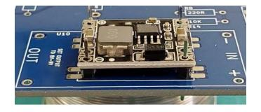
Place the buck converter on the pins
