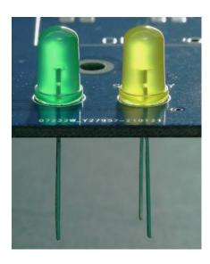
Try to get the LEDS flush to the PCB.
