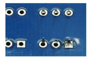
Solder a corner pin first then check the socket hasn't moved before soldering the remaining pins.
