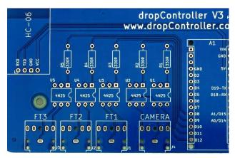
To help make assembly a little easier extra space has been added to the PCB layout. There are some tight spaces though; such as the pins on the Arduino and the IC sockets.
