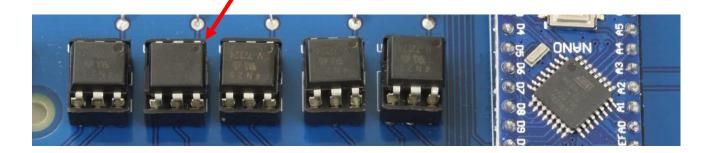
Make sure the pins are securely inserted in to the sockets and not bent.
