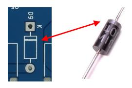
On the diode there is a white (it's actually grey or silver) line at one end, align this with the line on the PCB.
