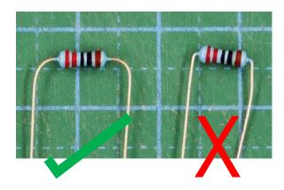
If you bend the pin too close to the resistor body you will find it doesn't fit the holes on the PCB very well, the resistor will want to sit at one end and will look messy.
