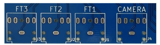
As with the optocoupler sockets, start by soldering one pin, check the position, then solder the other pins.
