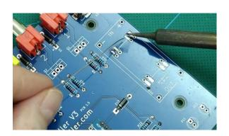
Tin the pads where the converter will go. Just need to add a small amount of solder.
