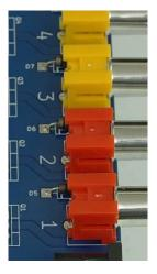
The phono sockets are another high stress part that benefit from a little more solder\*. Warm the pins and pads before adding the solder and let the solder run around the joint. Do not get it that hot that you melt the plastic and set fire to the PCB though.
