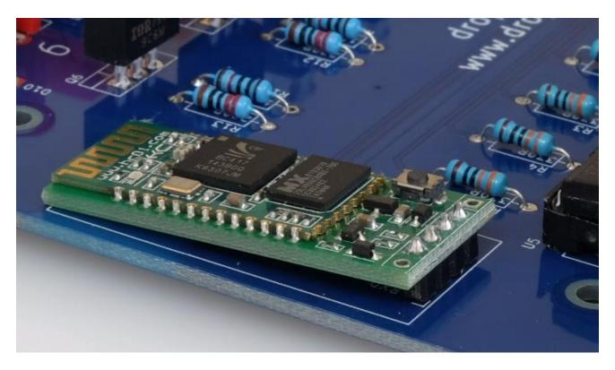
The Bluetooth module is at a slight angle so that the bottom of the board is against the PCB.
