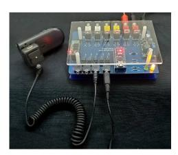
The camera is in manual mode, aperture set to F18, shutter set to 1 second. The flash guns are set to 1/64. The wireless flash trigger and the camera are connected to the dropController FT1 and CAMERA ports respectively.
