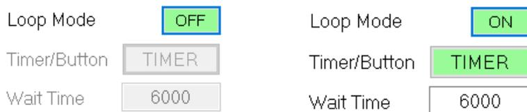
In Loop Mode there are 2 methods used to wait for the next sequence, either a timer or a button click.
