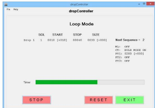
While the timer is counting down, clicking the STOP button pauses the app at the current sequence number. Click START to continue. To reset the sequence number back to 1 click the RESET button.
