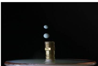
Make a drop and either move the focus aid to the impact position, or like me, move the bowl. Make another drop to confirm. If the drop hits the aid you are ok and can focus the camera on the focus aid.
