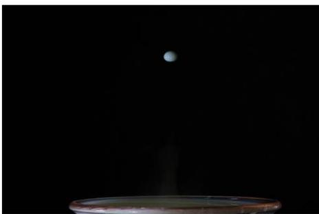
As it turns out 100ms wasn't a particular good place to start the flash trigger. I didn't see the drop until the flash trigger reached 350ms. This is not really a bad thing though and one of the main benefits of the dropController. With a manual system it would have taken a fairly long time to find what time the drop entered the frame. With the dropController you just use a delta value on the flash trigger, set the device going and monitor the images.
