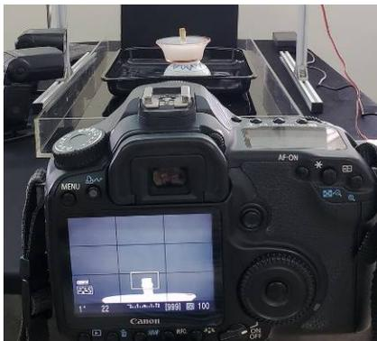
I am using a 105mm macro lens on a Canon camera and I have the camera level with the top of the bowl.
